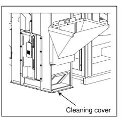
(6) Take off BUCKET ELEVATOR INLET BASE PLATE to drop the residual grain.
