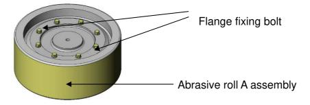
How to remove the Abrasive roll B is as well as Abrasive roll A. (This part is also heavy, so handle with care)
